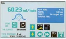
Run screen displays all operational parameters so you can confirm operation and program settings at a glance.
