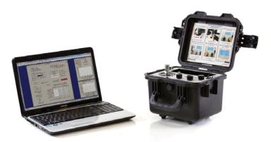
The Portable Accelerometer Calibration System, Model K9145D10, features accurate back-to-back comparison calibration of accelerometers in accordance with ISO 16063-21 (2003). A derivative of the industry-leading 9155 Accelerometer Calibration Workstation and based on a laptop PC system with a state-of-the-art 24-bit USB dynamic signal analyzer module, the K9145D10 offers a portable, turnkey calibration solution suitable for both laboratory and field portability.
