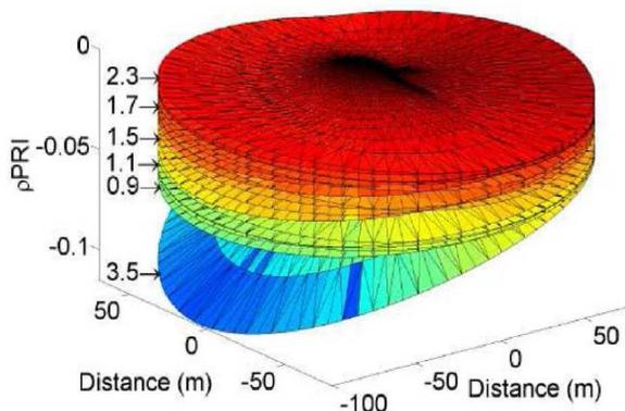
Fig 3: Bidirectional reflectance distribution model (BRDF) of multi-angular AMSPEC observations. The PRI reflectance observed is a function of directional and physiological reflectance effects of the canopy
