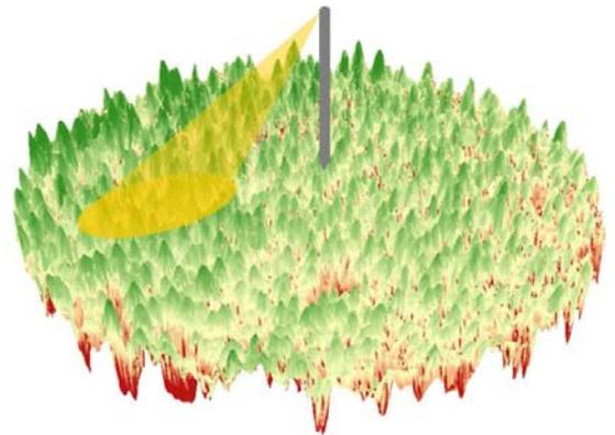
Fig 2: AMSPEC observes the forest canopy around the flux tower every 15 minutes; one scan is taken every 5 seconds. Data were collected over a one year period
