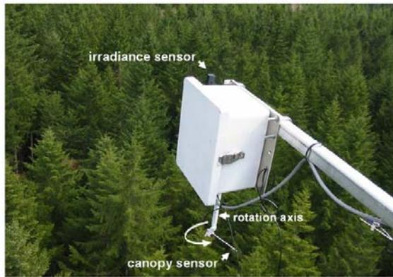
Fig 1: Multi-angular Spectroradiometer (AMSPEC) at the Research site near Campbell River (BC). The instrument is installed on a flux tower of the Canadian Carbon Program (CCP)
