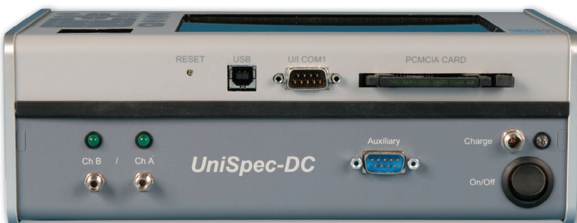
UniSpec-DC foreoptics interface (ChA/ChB), serial and USB ports, PCMCIA port, auxiliary connector and system power.
