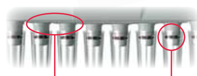
Stepped surface Sealing ring of FKM
