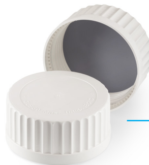
DURAN® PURE GLS 80® Screw Cap made from PSU with PTFE coated silicone seal
