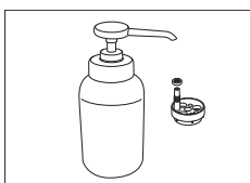
Rinsing unit with titration head insert, stoppers and manual dispenser.
