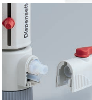
Valve system designed without seals
