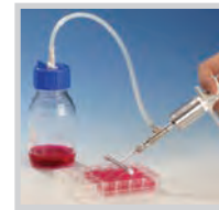
Aspiration with Reverse Modus Valve
