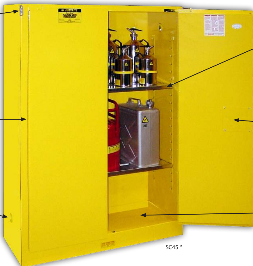
Fusible links hold doors wide open and melt at 74°C for automatic closure (1)
