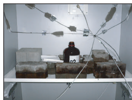
^Sensors in a flammable cabinet
