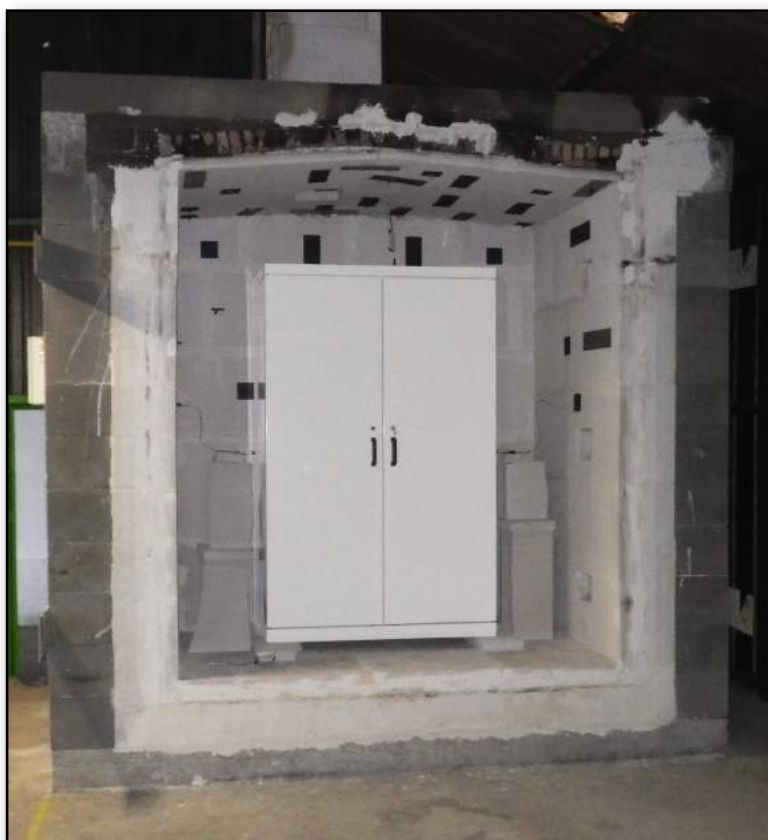
^795BG cabinet placed into the oven to fire test according to EN 14470-2 norm (photography before test).
