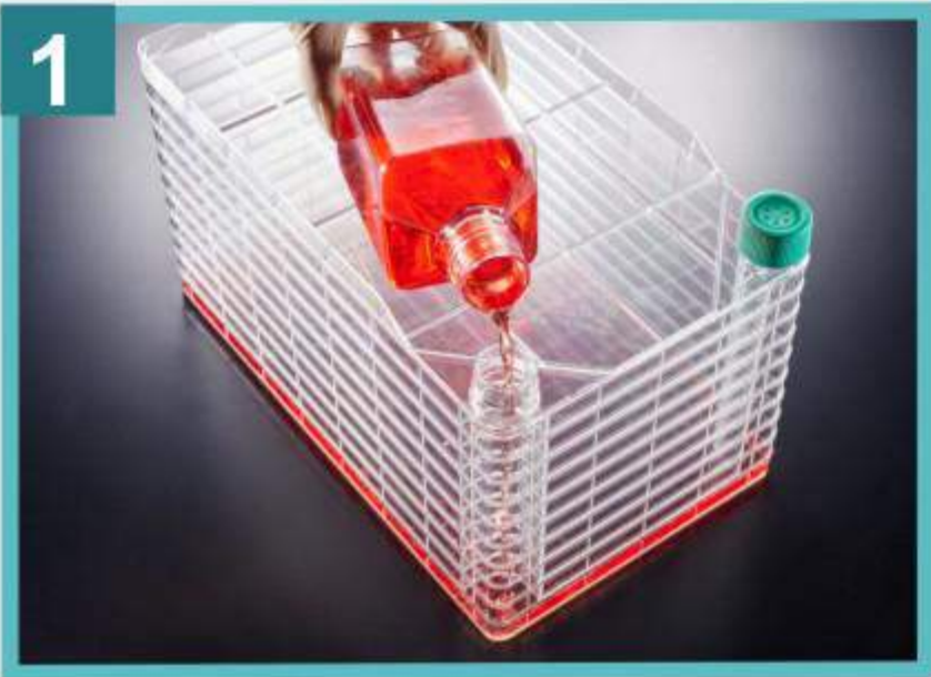
Pour the media directly into the Cell Factory system
