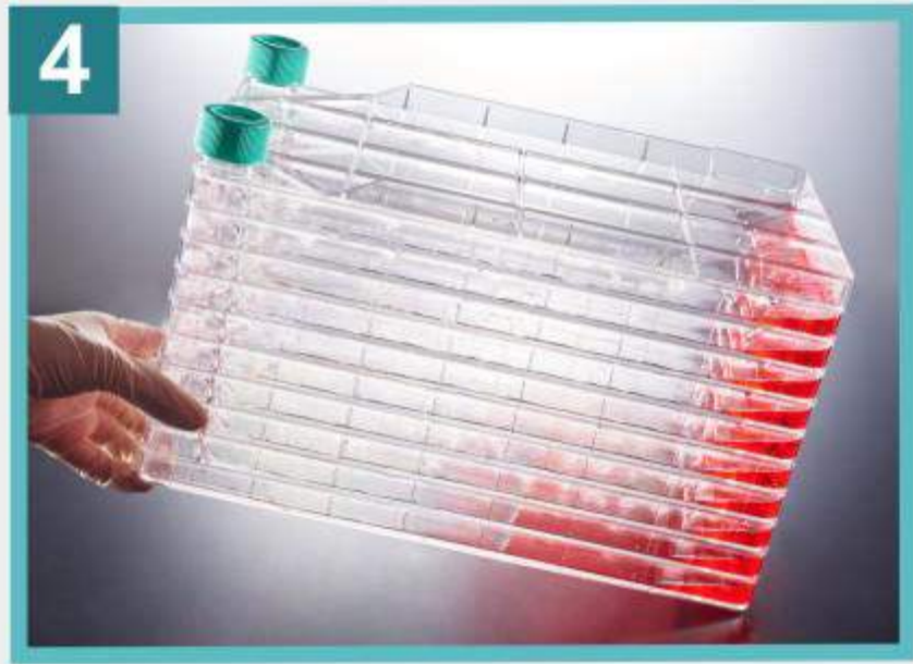
Carefully tilt the Cell Factory system to a horizontal incubation position with the filling inlet up
