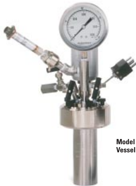
Model 4593 Reactor, Moveable Vessel, 100 mL, with PTFE Compression Gasket, and Split Ring Closure
