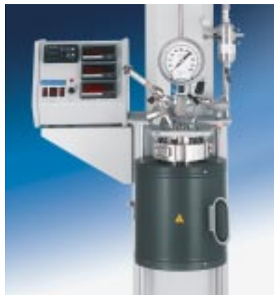
4534 Reactor, Assembled with Heater Raised
