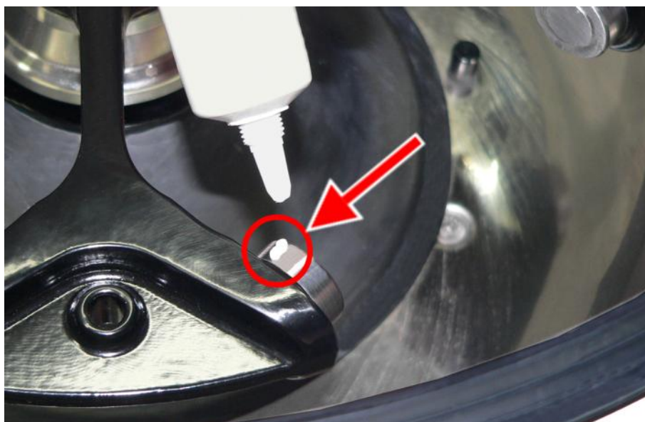
Fig. 16: Sufficient quantity of grease for one bolt
