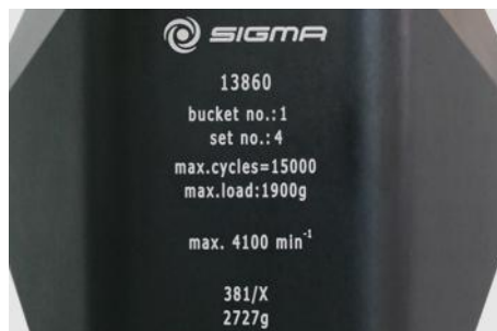
Fig. 4: Different service life – engraving on the bucket/rotor
