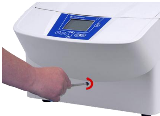
Fig. 15: Manual release of the lid lock
