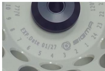
Fig. 4: Different service life – engraving on the bucket/rotor
