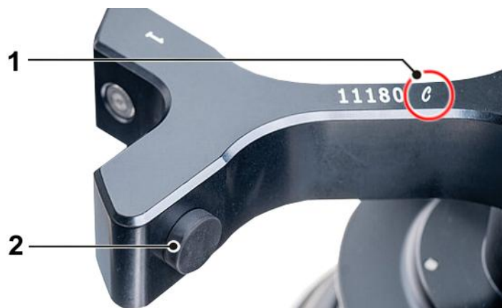
Fig. 6: Marking of a rotor with "Comfort" coating (example)
