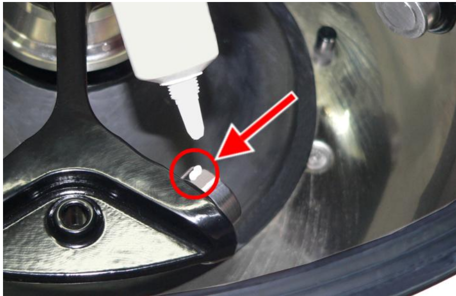
Fig. 38: Sufficient quantity of grease for one bolt
