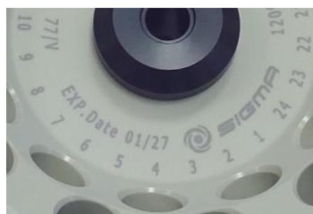
Fig. 7: Different service life – engraving on the bucket/rotor
