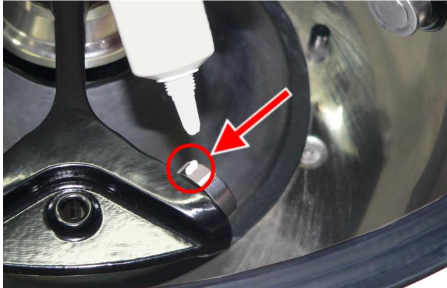
Fig. 37: Sufficient quantity of grease for one bolt
