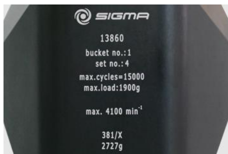
Fig. 6: Different service life – engraving on the bucket/rotor
