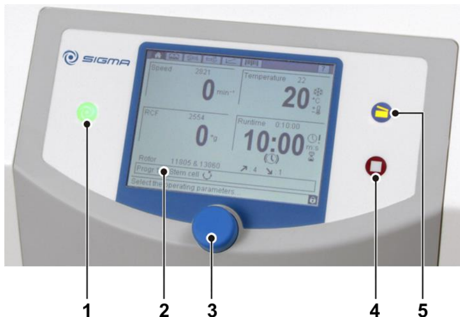
Fig. 15: User interface of the Spincontrol S control system
