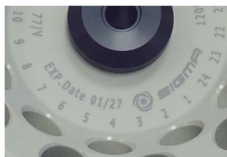
Fig. 5: Different service life – engraving on the bucket/rotor
