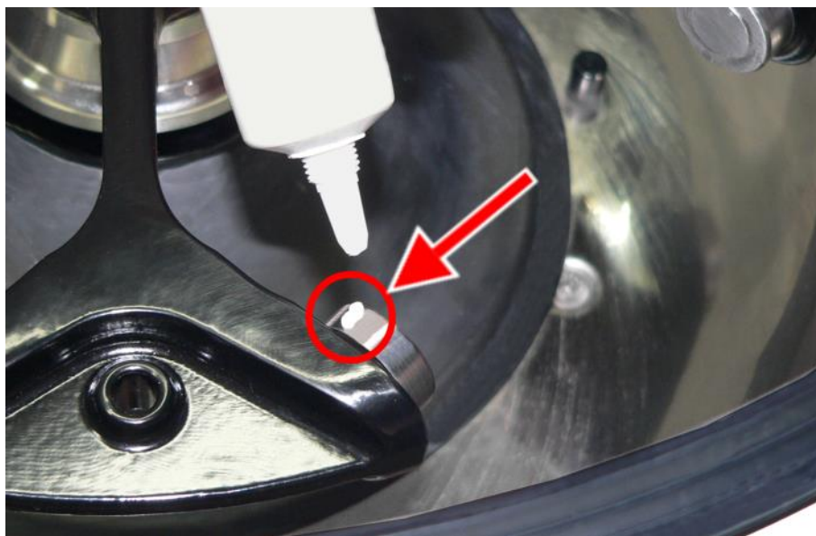
Fig. 37: Sufficient quantity of grease for one bolt
