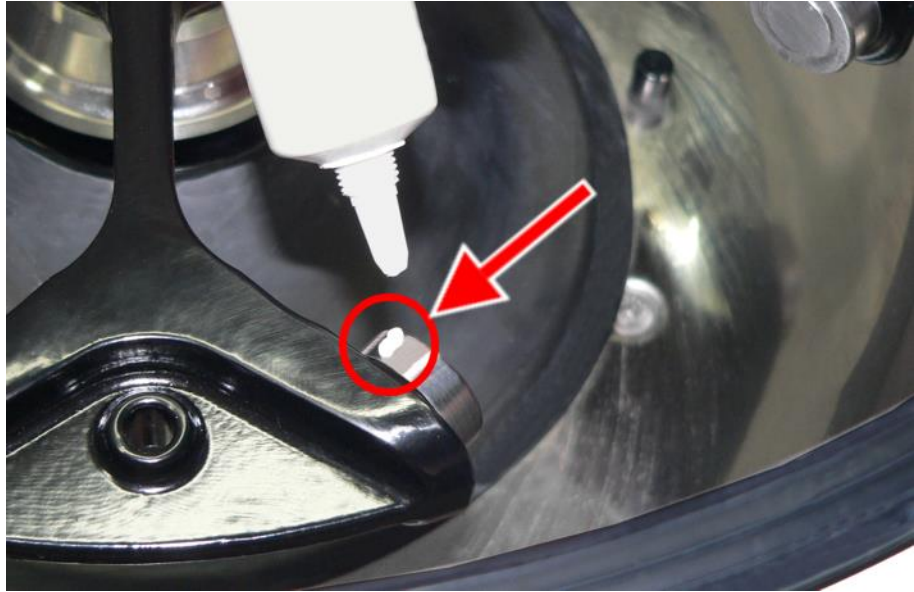
Fig. 38: Sufficient quantity of grease for one bolt
