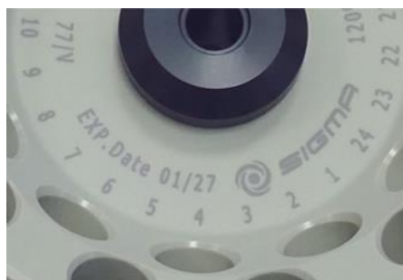
Fig. 6: Different service life – engraving on the bucket/rotor
