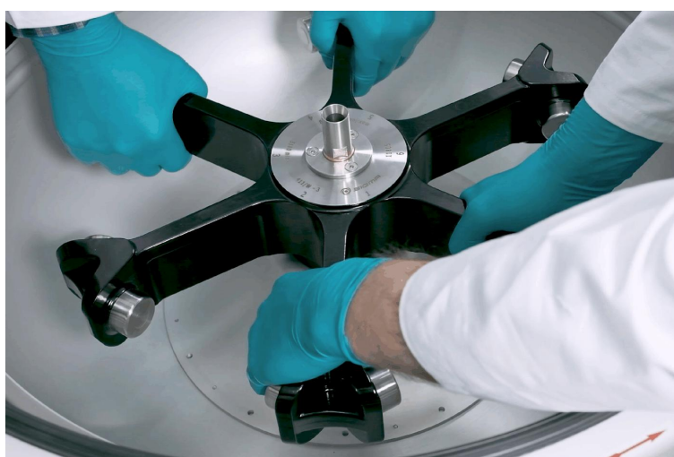
Fig. 18: Correct method for lifting the rotor 11805 with a windshield
