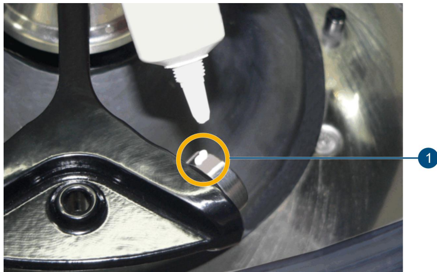
Fig. 42: Applying the grease for load-bearing bolts
