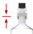
Ground joint stuck
