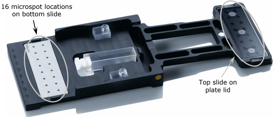
Figure 2: Plate open, showing slides and "microspots"
