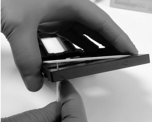
Figure 5: Using a pipette tip to remove a slide
