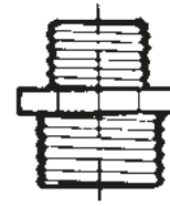
Nipple, reduced, with outer thread.
