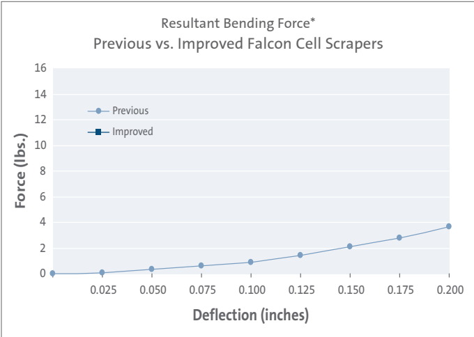
Force required to deflect a simply supported 5" portion of the handle 2.5" distal to the handle section: resultant = ('X' force) ('Y' force).
