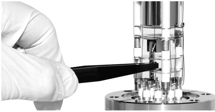
Figure 5 Remove the Electron Multiplier
