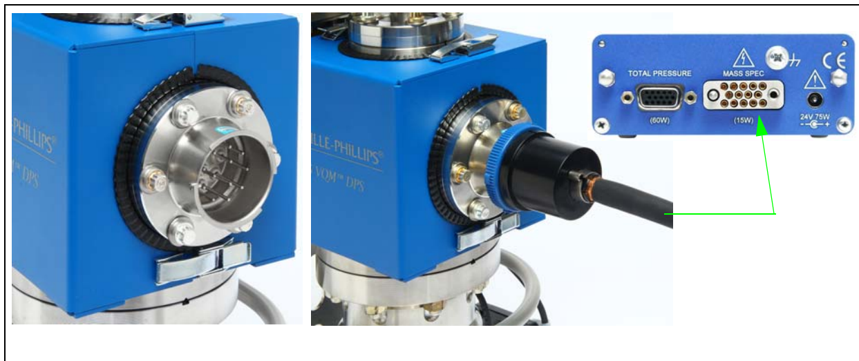
Figure 3-3 Cable Connections - MS Gauge to VQM Controller
