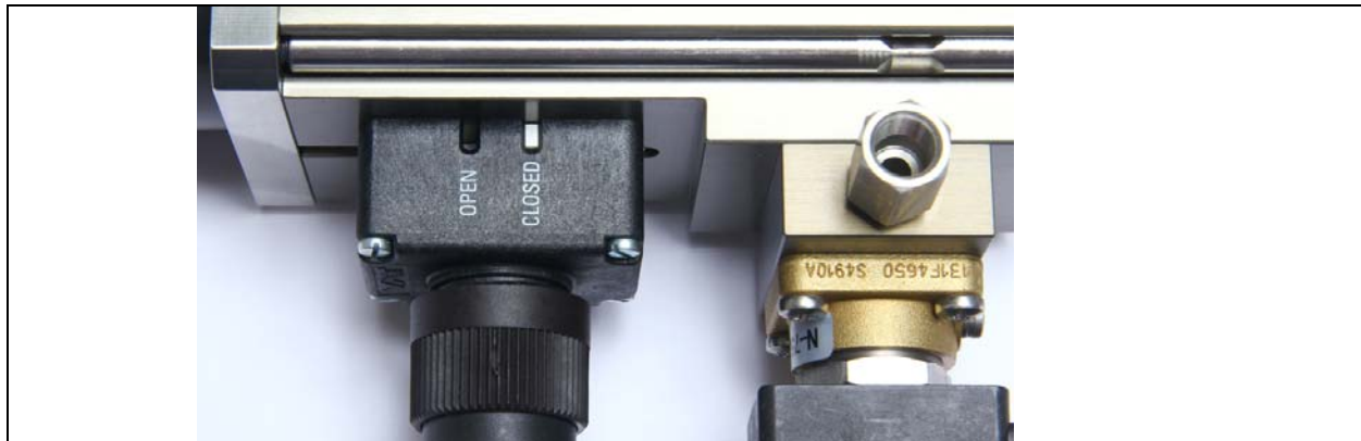
Figure 3-8 Gate Open/Closed Visual Position Indicator
