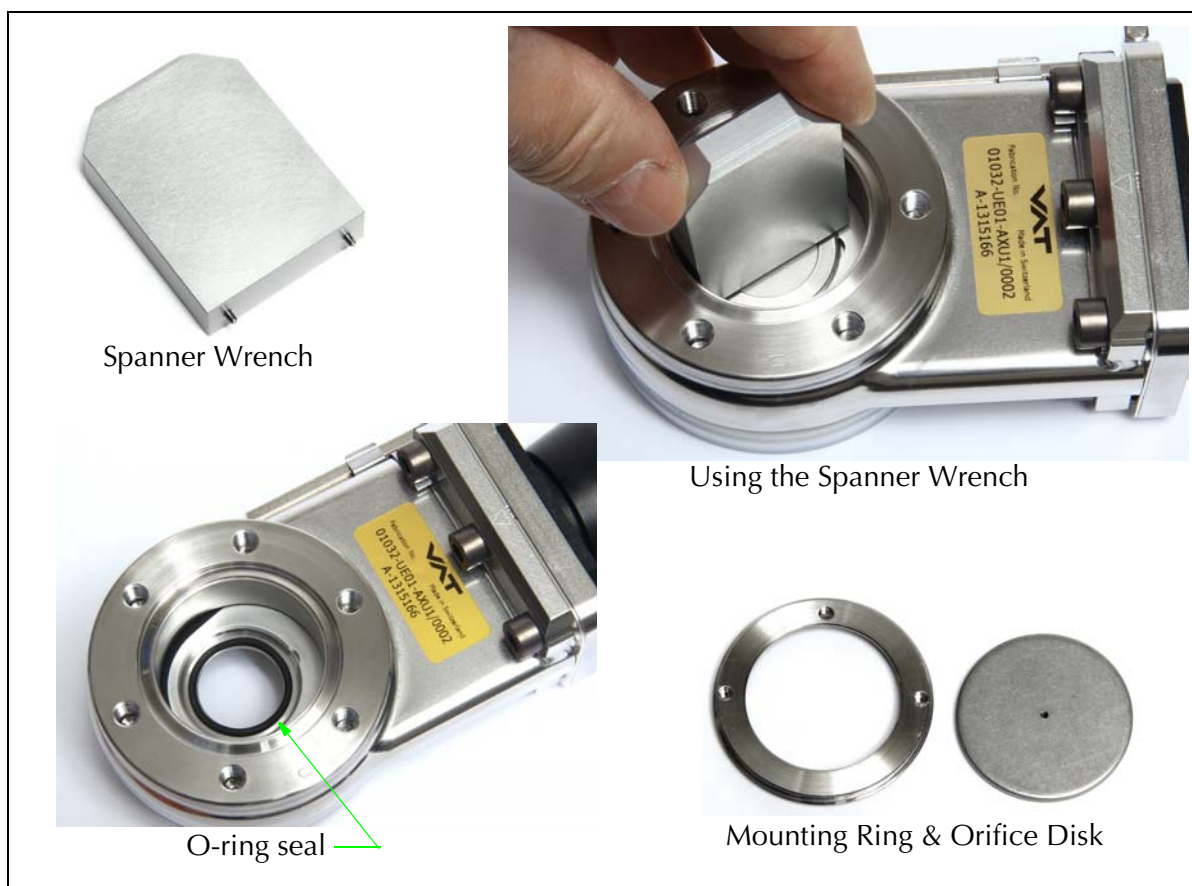
Figure 5-3 Orifice Disk Replacement (valve shown removed from the system)
