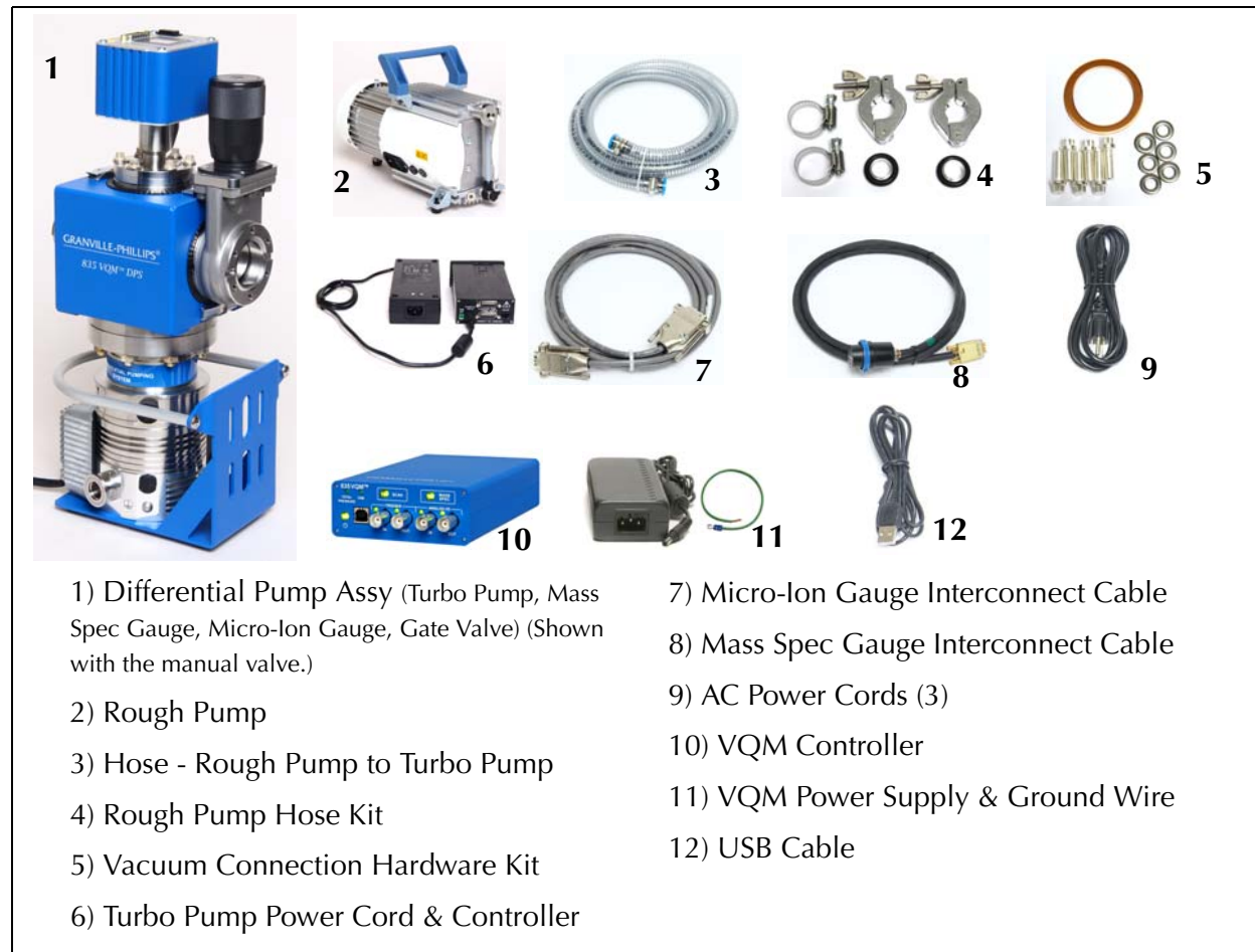
Figure 2-2 Components of the VQM Differential Pump System
