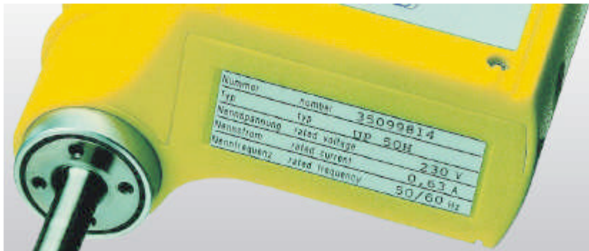
Figure 4-4 Rating plate of an ultrasonic processor UP50H (electric connected loads are country-typical)
