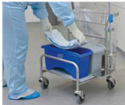
2 Load the system box with no more than 12 mops – ensure that the back of the mop (pocket) is pointed up
