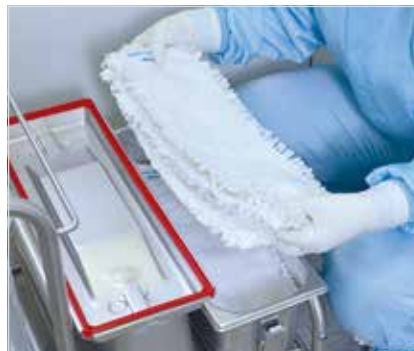
2 Load the system box with no more than 10 mops – ensure that the back of the mop (pocket) is pointed up
