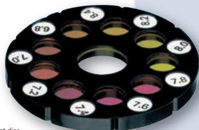
Test disc with colour stable glass standards
