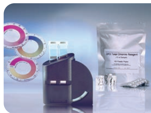
CHECKIT® Comparator with powder reagent / tablets
