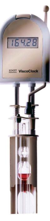
For temperature stabilization in the thermostatic bath, the following tempering liquids are suitable: water, alcohol water (e.g. ethanol, methanol), paraffin oil, and silicone oil. Liquids can be measured that qualify for use with the viscometer being used in each instance.
