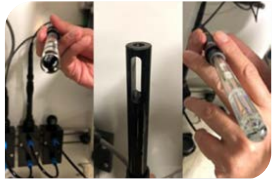
Fig. 3: Sensors after five months of operation (Left: oxygen sensor, center: conductivity sensor, right: pH sensor)
