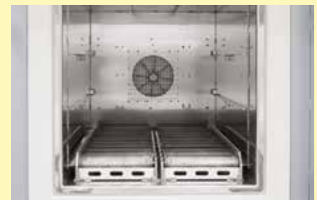
Roller conveyor in furnace chamber
