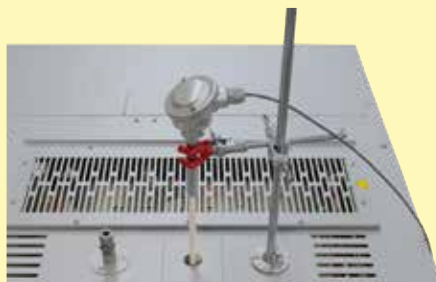
Thermocouple port in the ceiling with tripod
