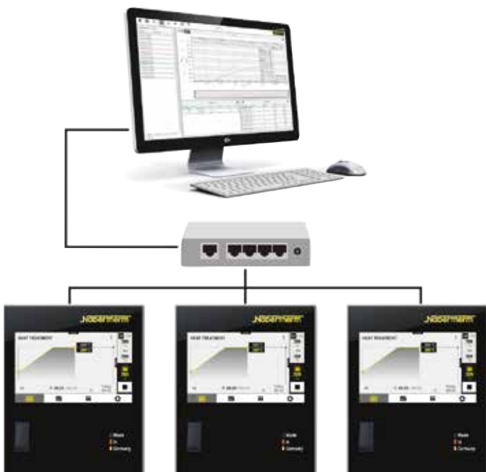
Example lay-out with 3 furnaces
