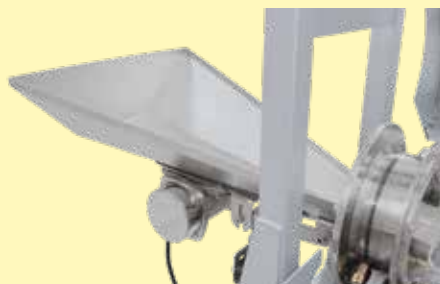
Vibrating channel on the rotary tube for convenient material feeding
