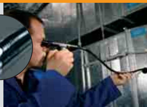
Inspects air duct, with gooseneck casing, middle flexibility
