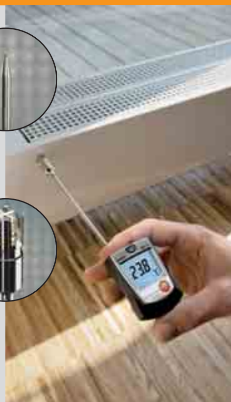
Checking temperature on a radiator
