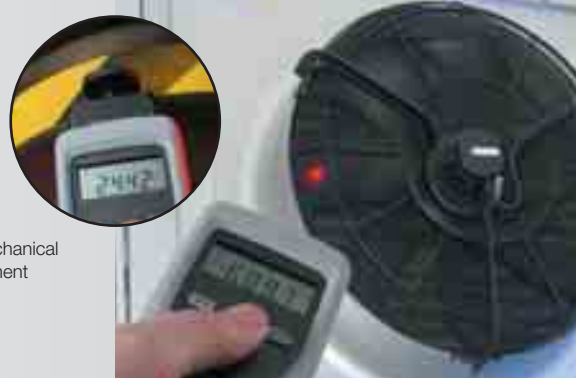
testo 465 and testo 470, non-contact (optical) rpm measurement on rotating parts
