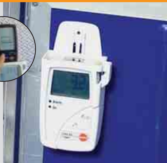
Long-term temperature logging with immediate display of limits exceeded
