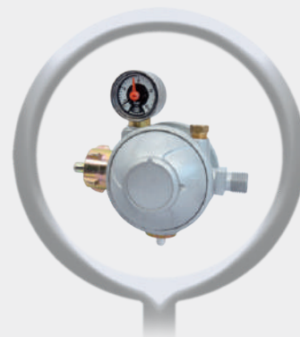
DVGW low pressure regulator DIN 4811-4, for household liquid gas installation, with overpress., temperature- fuse & manometer, for gas bottles up to 14 kg Art.-No. 6.000.150
